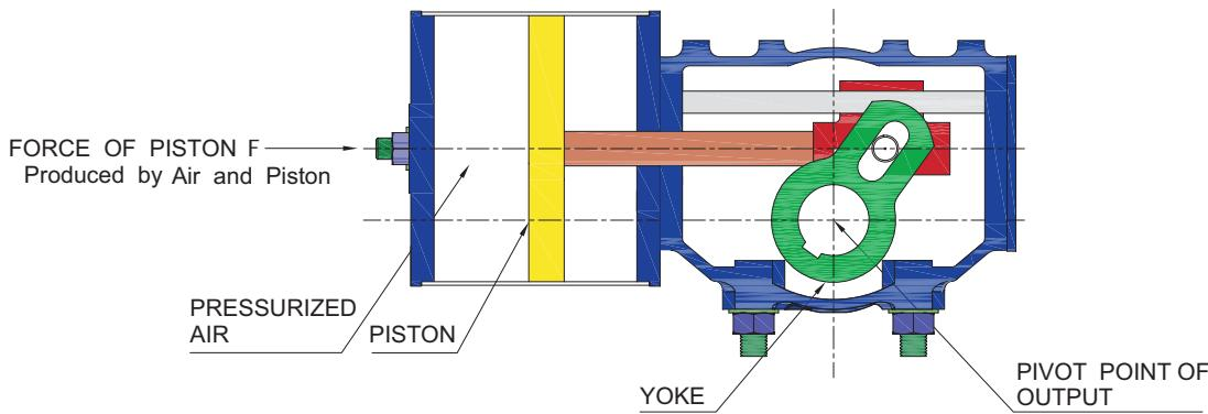
THE SCOTCH YOKE ACTUATOR IS A LINK MECHANISM ON A SWEEP OF 90°
