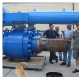
20" ANSI 2500 Trunnion w/ butt weld ends and pipe extensions
